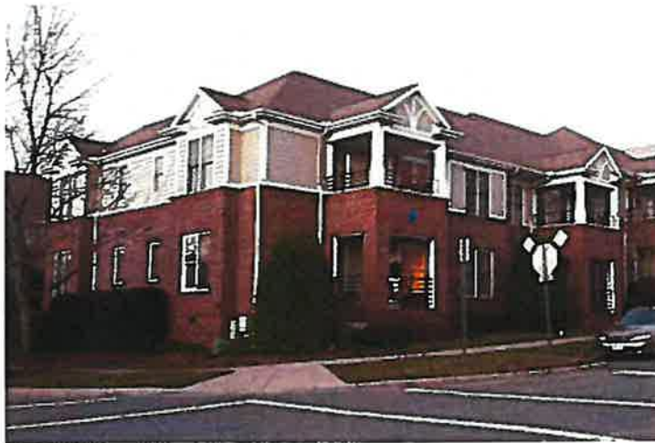
Figure 6-7-10: Heavier materials below lighter elements
